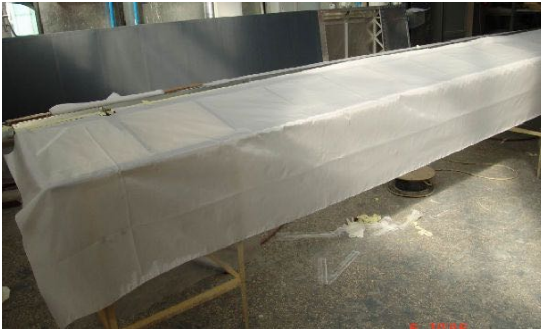
Photo 18 (for all components except for elevator and wing the fabric is pre-cut to overlap both sides)
